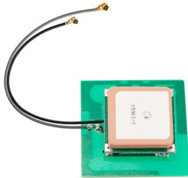
An embedded GPS Antenna and cellular module.
